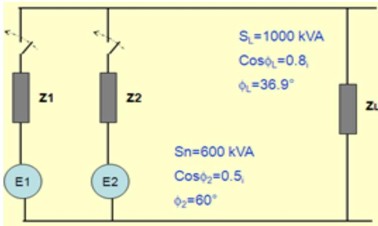
$$\bar{S}_2 = 600 \angle 60^\circ = 300 + j520 = (P_2 + jQ_2) \text{ KVA}$$
