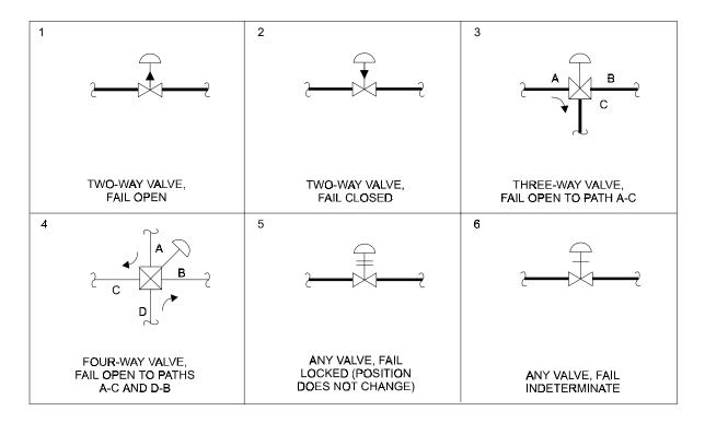
The failure modes indicated are those commonly defined by the term, "shelf-position." As an alternative to the arrows and bars, the following abbreviations may be employed:
