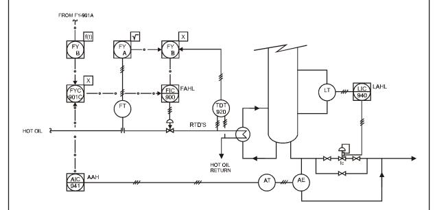
DETAILED SYMBOLISM AND MORE COMPLETE IDENTIFICATION USED TO DESCRIBE THE CONTROL SYSTEM WHEN TYPE OF HARDWARE AND KINDS OF SIGNALS HAVE BEEN CHOSEN.
